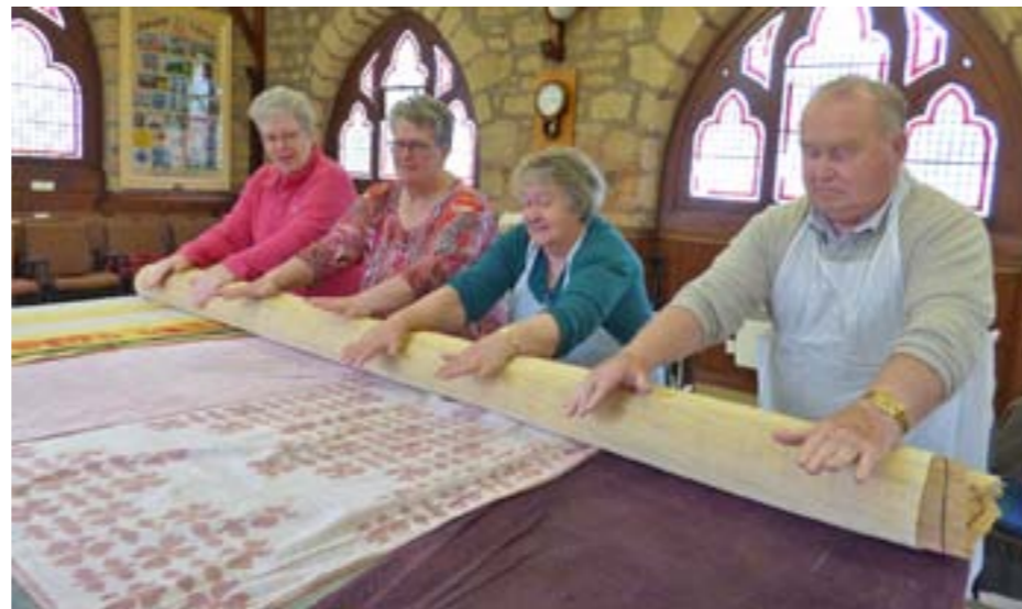
This rolling process is called milling and it firmed up the felt, shrinking it each time in the direction of rolling.
